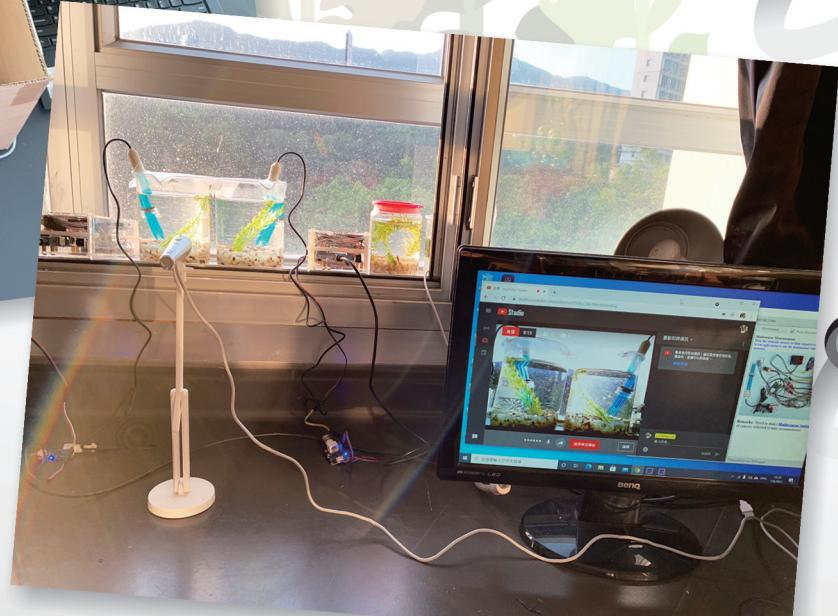
The remote laboratory investigating the gas exchange of aquatic organisms in the ecospheres under different conditions
