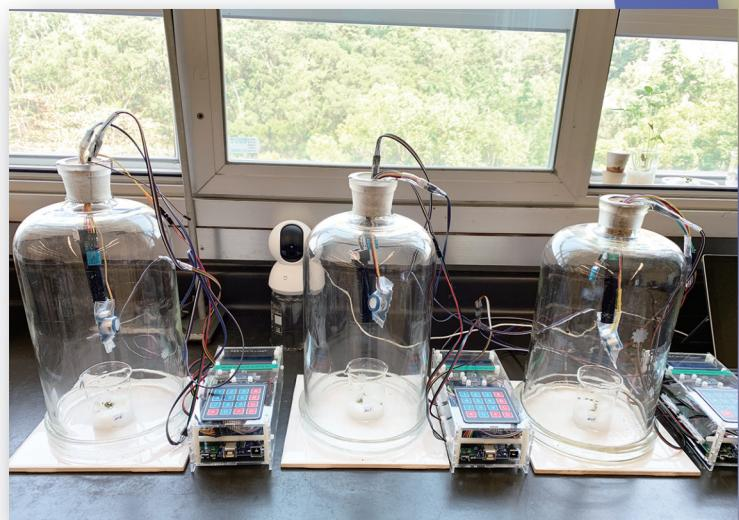
Set-up of the Arduino mobile datalogger for a POE activity in our science laboratory
